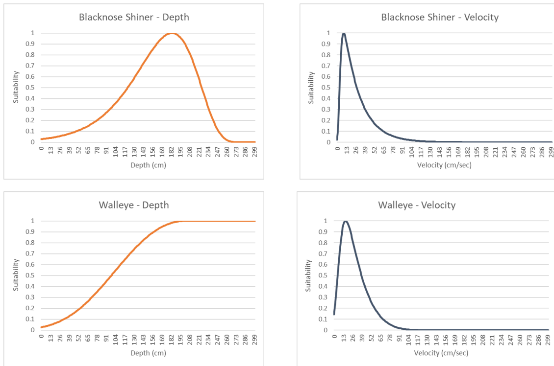
FIGURE 9 (CONT.). HABITAT SUITABILITY CURVES FOR DEPTH AND VELOCITY OF THE 10 MOST COMMON SPECIES IN THE GILE FLOWAGE MINIMUM FLOW HABITAT EVALUATION STUDY REACHES.
